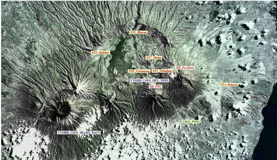
*Kawah Ijen seismic network (Blue and Green: USGS and CVGHM seismic stations / Red and pink: ROB seismic stations, respectively short period and broadband sensors)*
