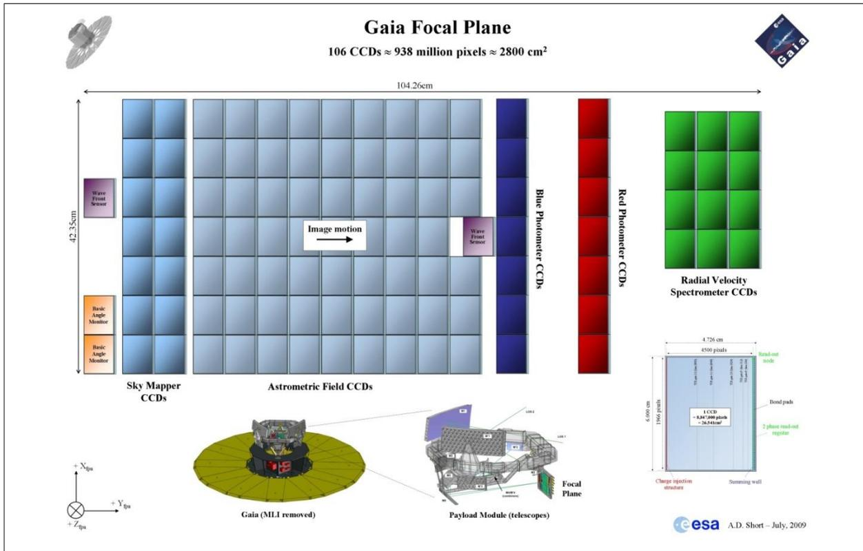
*The Gaia focal plane will be the largest ever developed, with 106 CCDs, a total of almost 1 Gigapixels and physical dimensions of 0.5m × 1m (Image credit: ESA - A. Short)*
