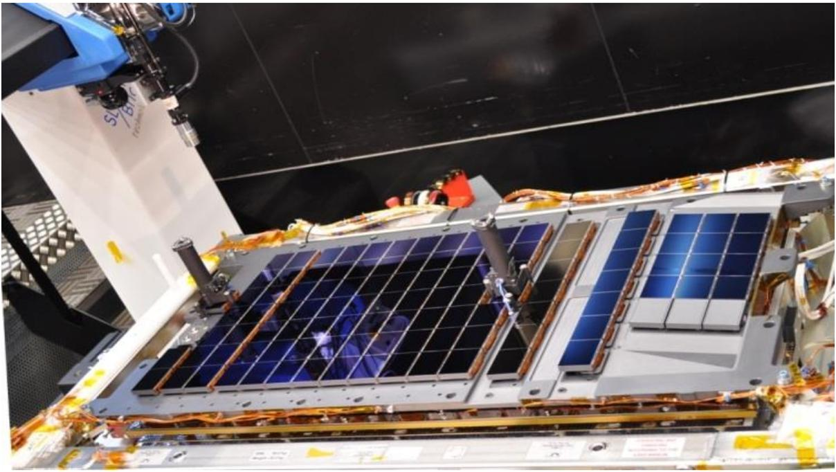
*The complete set of 106 CCDs that make up Gaia's focal plane was assembled in 2011 (Copyright: ESA/Astrium)*
