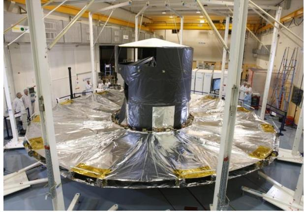
*Gaia Deployable Sunshield Assembly (DSA) in 2011 fully deployed at Astrium Toulouse (copyright Astrium)*
