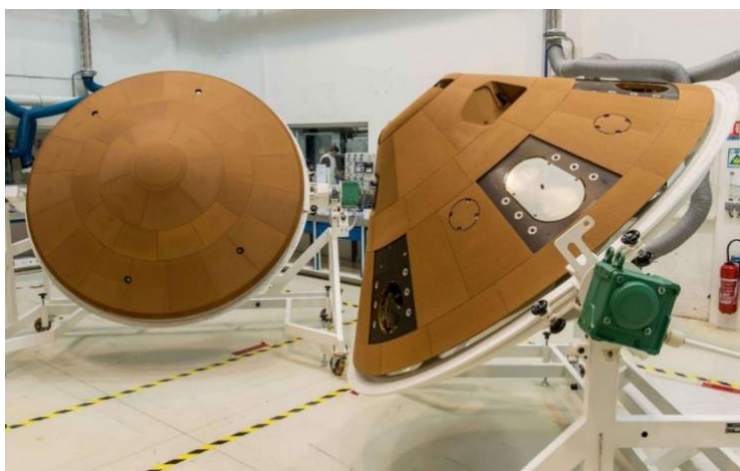
ExoMars 2016 EDM: heat shield (left) and back shell (right) from Airbus Defense & Space (image credit: ESA).
