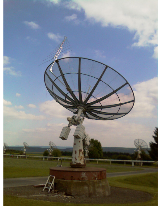
Figure 47: the new 50-1300 MHz log-periodic antenna mounted on the outer ring of a refurbished 6m parabola.
