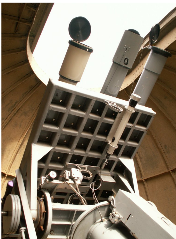
Figure 51: View of the underside of the Equatorial Table, showing the small pointer telescope with the sensor unit (4-quadrant photodiode) and electronic box.
