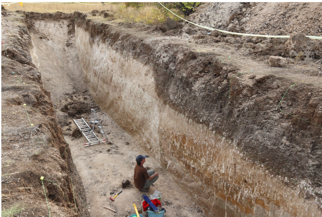
Figure 26: Overview of the west wall of Tatarevo trench 3. The fault is situated in the middle of the trench, and clearly displaces the uppermost black soil unit
