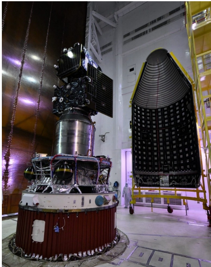
Figure 1: The two PROBA-3 spacecrafts are seen mounted on top of the upper stage of the PSLV-XL launcher, in one of the last photos taken before the rocket fairing has been closed, Satish Dhawan Space Centre, Sriharikota, India, 29 November 2024.
