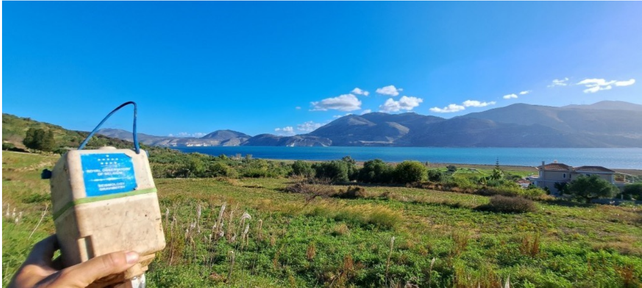
Figure 21: Installation of SmartSolo geophones on the Paliki Peninsula, Kefalonia, Greece. Credit: ORB-KSB.
