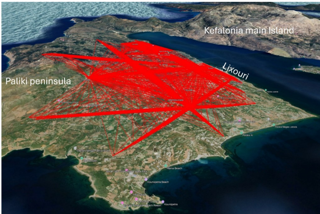
Figure 23: Raypaths between simultaneously installed geophones crossing the town of Lixouri and the Paliki Peninsula. Credit: ORB-KSB/MNCN.
