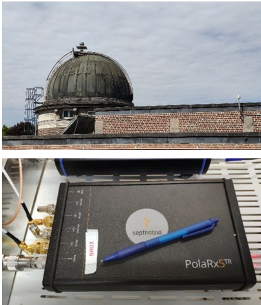
Figure 33: antenna and receiver connected to the atomic clock at the Royal Observatory of Belgium, measuring the GNSS satellite signals. These measurements are then analysed by the Atomium tool for time and frequency comparisons with the clocks of other laborator. Credit: ORB-KSB.
