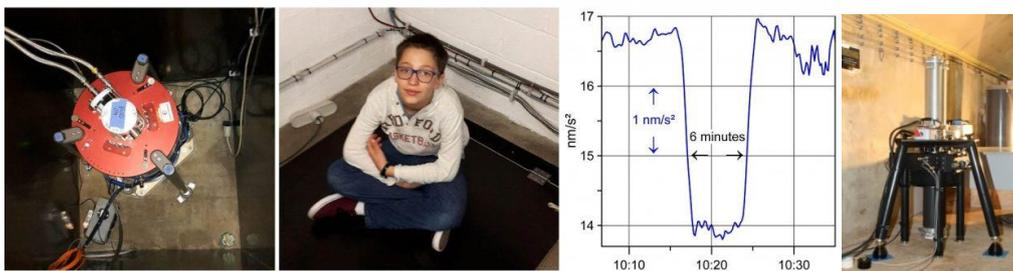
**Left: The relative superconducting gravimeter installed in a shaft at the Rochefort station, Belgium. Center-left: A 13-year old boy, weighing 45 kilograms, sat with his navel 1 meter above the instrument. Center-Right: The gravitational effect of the boy sitting for 6 minutes: his mass induced a decrease in gravity of 0.28 billionth of g. Right: the FG5 absolute gravimeter measuring at the Membach station**
