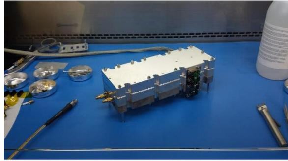
Flight Model of the transponder while mounting the PCBs. Three PCBs are already mounted
