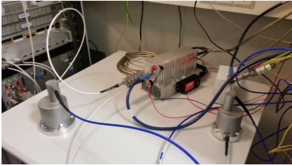
The LaRa transponder and antennas (covered with a cap) at ESOC for performance testing
