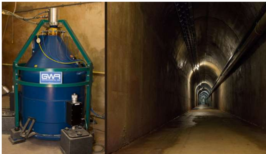
Figure 2: The superconducting gravimeter is located at the end of a 132 m – long gallery, 48 metres underneath the surface, in Membach (city of Baelen, eastern Belgium). The instrument sensor is immersed in liquid helium in which the temperature is held at -269^{\circ} , in other words, 4 degrees above absolute zero, allowing superconductivity. Photo credit: E. Coveliers & B. Frederick. Copy authorised with mention of the source
