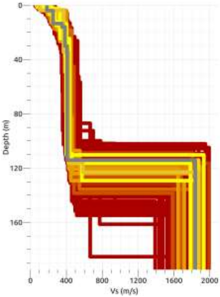
Figure 13: One of the main site-characterisation products, showing a shear-wave velocity ( v_s ) model with depth for the seismic station in Uccle at the ORB-KSB.
