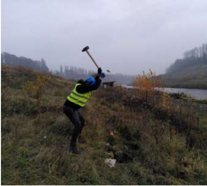
Figure 12: Site-characterisation fieldwork in Seneffe (SNF), using seismic waves excited through hammer shots to analyse the subsurface structure in the vicinity of the seismic station placed in a shallow borehole next to the little building in the photo.
