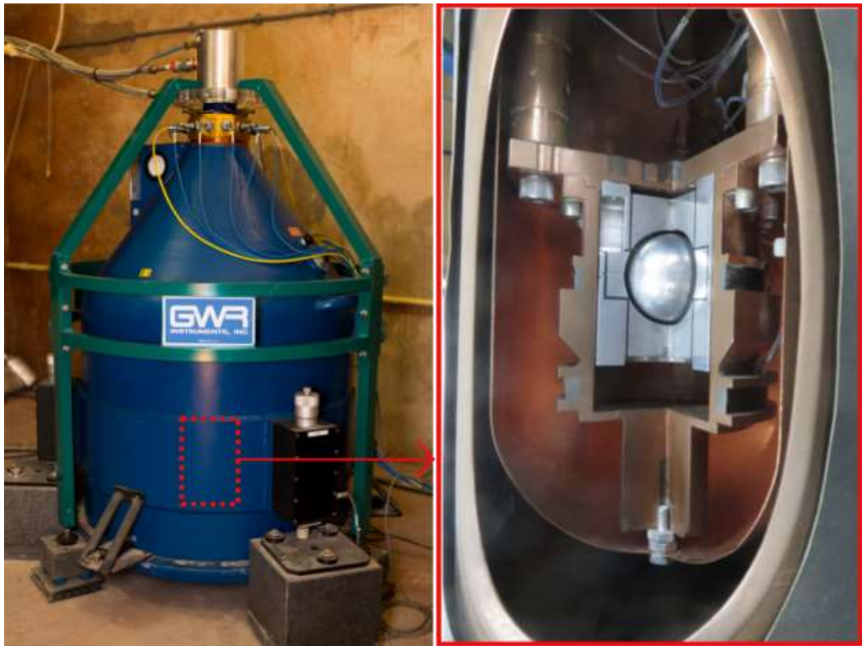
Figure 12: The Membach's superconducting gravimeter and an exploded view of the sensor with the levitating sphere. Left photo: E. Couveliers.
